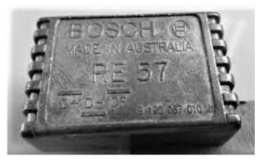
On the left is a photo of the Bosch RE57 voltage regulator, packaged in a small die-cast case. It is a sealed, non-adjustable three-terminal (D+, DF, D-) device which provides an install-and-forget solution. It has a voltage set point of 14.2V. More follows. The regulator's metal case is a heatsink, so mount the unit firmly on the firewall.
