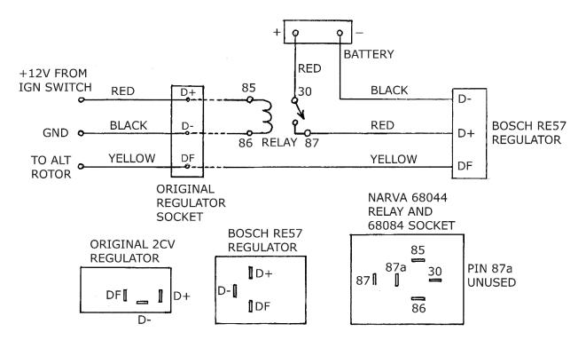
PIN DESIGNATORS ARE SHOWN WHEN LOOKING DIRECTLY AT THE PINS
