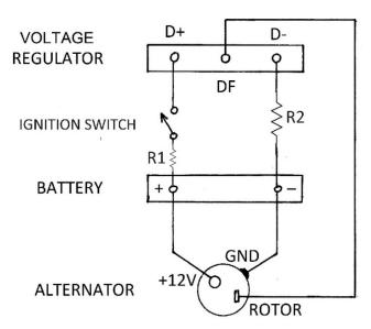
We will consider the 2CV battery charging circuit shown in the writer's article, *2CV Battery Charging Circuit*. We'll add to the circuit the critical wiring resistances, shown as resistors R1 and R2 in the figure above. Resistor R1 represents the wiring resistance between the voltage regulator's D+ terminal and the battery positive post via the ignition switch, and resistor R2 represents the wiring resistance between the regulator's D- terminal and the battery negative post.
