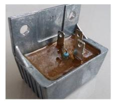
original regulator socket if necessary. Alternatively, the socket could be removed and the wires extended. The D+ and D- wires connect to the relay coil while the DF wire connects to the DF terminal on the RE57 regulator. Note that relay pin 87a is not used. The colours of the three wires at the original regulator socket may vary and sometimes they are all the same colour! Photograph, trace, label and record the socket wiring details very carefully and keep the information in a safe place.
